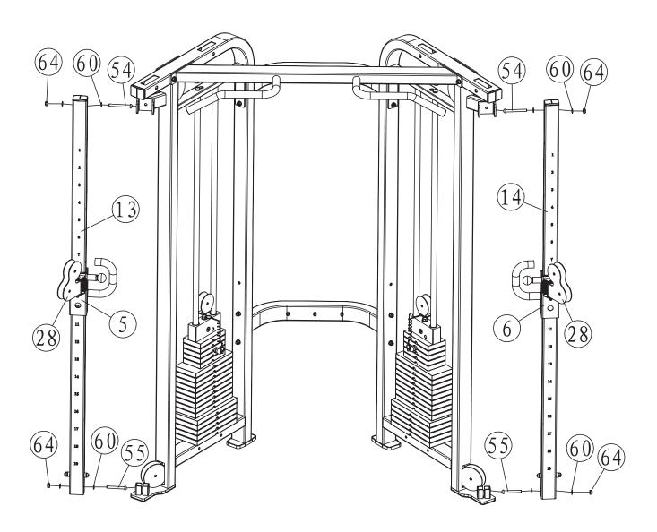
**STEP 4** Slide Left Frame Slip (5) onto Left Slip Tube (13).
